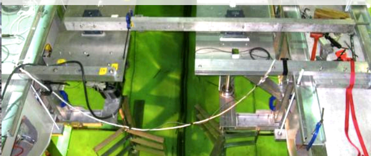
Performance testing of twin hydrokinetic turbines in a towing tank at National Research Council of Canada
