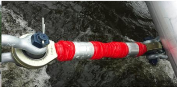
Submersible load cell with integrated data recording
