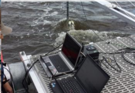
Current measurements using ADCP deployment off custom boom
